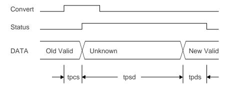
DATA refers to both the data and over-range signals. The Convert pulse can be any width, including zero. If the propagation delay between the rising edge of the Convert signal and the Status signal (tpsd) is zero, the data and over-range do not go to unknown but directly to the new value. There is a resistive load from <ref node> to <gnd node>, and from <in node> to <gnd node>, of 1/GMIN.
